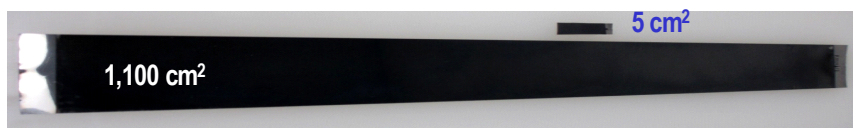
Figure 5. Successful scaled replication of CIS absorber deposition on 5 cm 2 and 1,100 cm 2 foils
